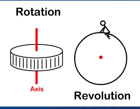
The difference between rotation and revolution is the location of the axis of rotation. The Ferris wheel turns about an axis. The Ferris wheel rotates, while the riders revolve about its axis.
